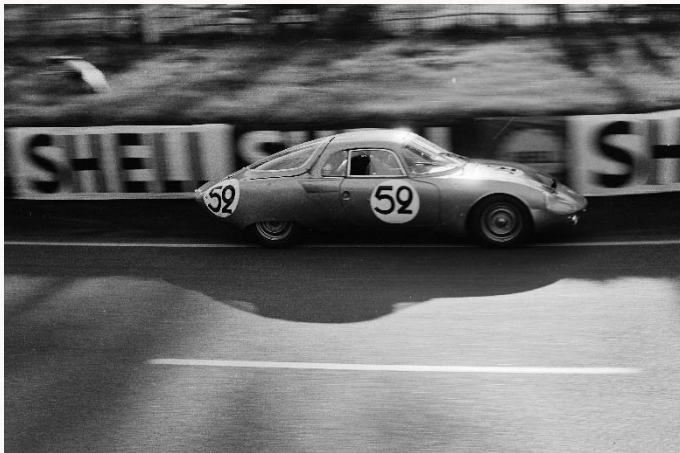
Alpine M63 powered by 93hp Gordini engine – first racing car from Dieppe
